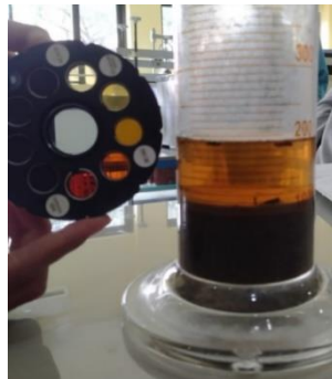
Gambar 1. Hasil Pengujian Kadar Organik Agregat Halus
